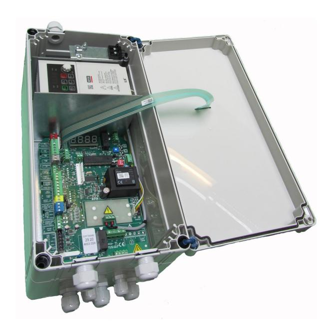
The frequency converter control generated various frequency which allows soft starting, soft stopping and various speed in up and down direction. Soft start and soft stop protect the door mechanism. Fast speed for opening and closing save building energy.
